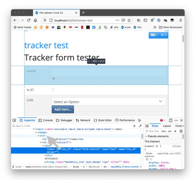
This form is a simple wiki table, so the container element is the tr (table row) which contains the input and the label, so your selector will be simply tr, but to make sure it doesn't get confused if the table's inside another one use tr:first, so your markup should be:
